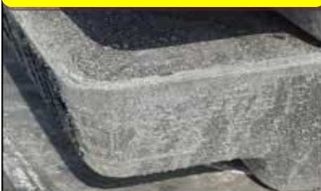
Severely corroded/oxidized sow
