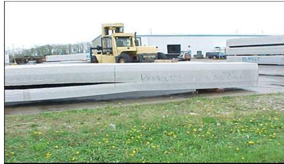
Unsafe Crack for Ingot Handling
